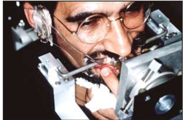
Fig. 7 In vivo friction test. 6 Maxilla is fixed in custom-cast splint, leaving mandible free. Testing machine pulls straight wire with preadjusted angulation and inclination through bracket on central incisor of spaced dentition. Whenever patient occludes, friction is immediately and markedly reduced.
